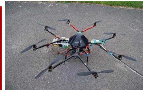
Octocopter - the first platform by Max Planck Institute for Biogeochemistry, Jena, Germany tested a measurement sensor package for air quality
